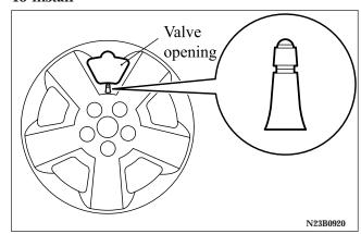
Align the air valve with the valve opening provided on 8 the wheel cover.
